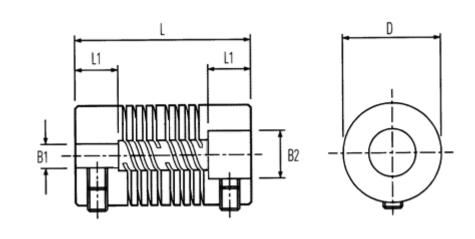
B1: Pre-drilled= 4.8B2: Pre-drilled= 6.35D= 19.1L= 28.0L1= 6.5Max angular displacement= 0.25Max B1 & B2= 10.00Max parallel displacement= 7
